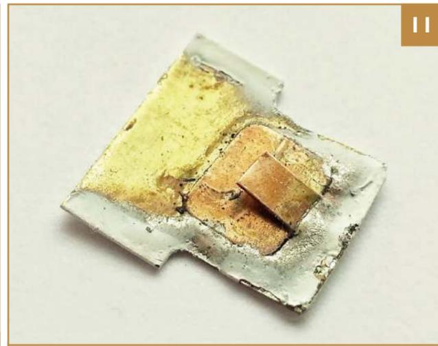
**11.** Cut the T shaped rear as per the picture and solder a small contact on the inside made from phosphor bronze strip.
