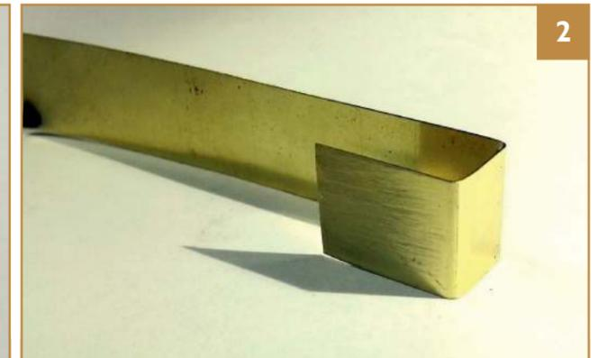
2. Take the strip and bend it into a 'u' shape with two 90 degree corners as shown in the photo. This will make the front and sides of the lamp, the folds should leave you with a front measuring 9mm wide, cut the sides to approximately 14mm length. These are oversize, but it's best to trim the lamp down when completed.
