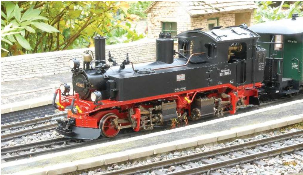
**Left – Front ¾ view:** Another posed picture with the loco blowing off furiously. The tank filler hatches lift, the fireman's side gives access to the water top-up point and the driver side hatch gives access to the switches to turn the head and tail lights on and off (one switch for on/off and the other for front/rear). The cab roof lifts off rather than being hinged – a squint through one of the half open roof vents enables you to read the pressure gauge.
