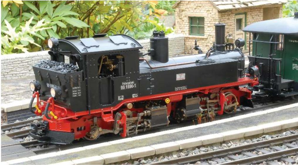
**Left – Rear ¾ view:** The leaf springs on which the rear bogie wheels ride are visible in this picture. I reinforced them as the loco originally rode too low at the back. The cab steps do limit the swing of the rear bogie but it will happily go through 5' curves without fouling. The additional coal capacity provided by the wooden extension is removable giving access to the receiver. Finally, the lubricator drain can be seen below the footplate above the lifting arm of the rear bogie.
